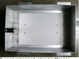
Support grid properly placed in filter pan.
